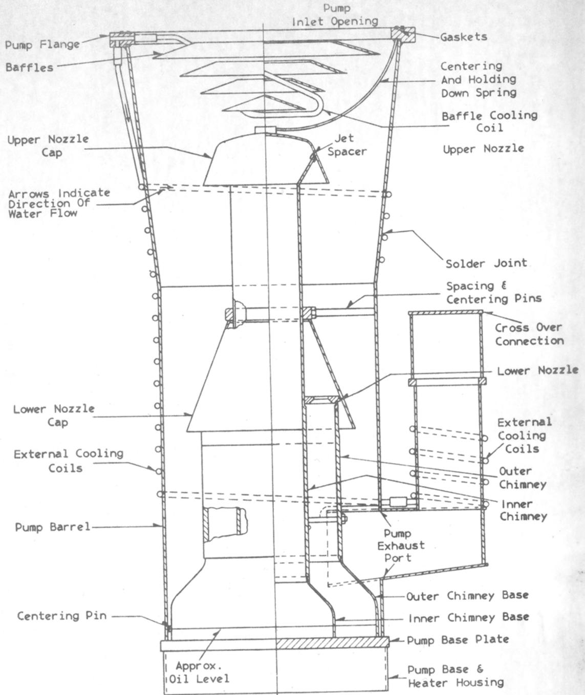
Cross-section of a 20-Inch Oil Diffusion Pump
