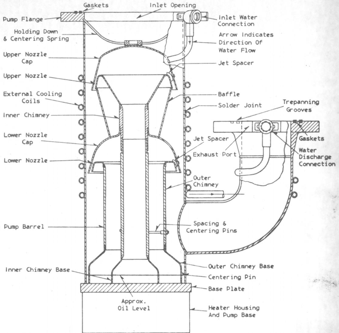
Cross-section of an 8-Inch Oil Diffusion Pump
